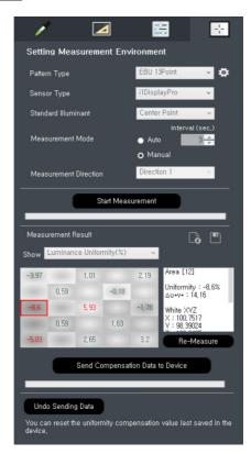
The screen's [Uniformity Compensation] feature is supported for OLED Pro models, which are for image quality professionals. This feature enables users to increase screen uniformity. In order to use this feature, the program and the OLED Pro product must be connected, and the PC with the program installed must be connected to the calibration sensor via USB.
