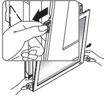
3. Push and close the top part of the front panel and then pull the bottom part of the panel forward until it is secured.
