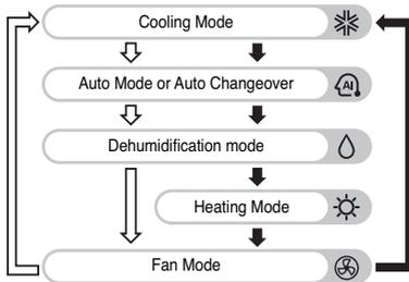
• Cooling model(↓), Heat pump model(↑)
