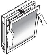
2. Pull out the both links of lower part of front panel, as described in the below picture.
