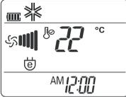
Energy-saving cooling mode can save energy in cooling operation, because it can operate efficiently by setting body-adaptation time according to the change of time and temperature and adjusting desired temperature automatically.
