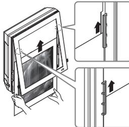
9. Push both links of lower part of panel inside and fix it. Then turn on.
