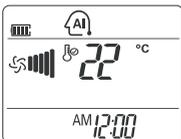
This operation is basically heating or cooling function of the air conditioner. But during this operation the controller changes the operation mode automatically to keep the temperature within  $\pm 2^{\circ}\text{C}$  with respect to the setting temperature.
